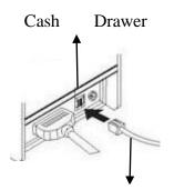
Use 12-24V/1A power supply cash drawer, which is also compatible with printer. The improper cash drawer will cause damage both to the cash drawer and the printer.
